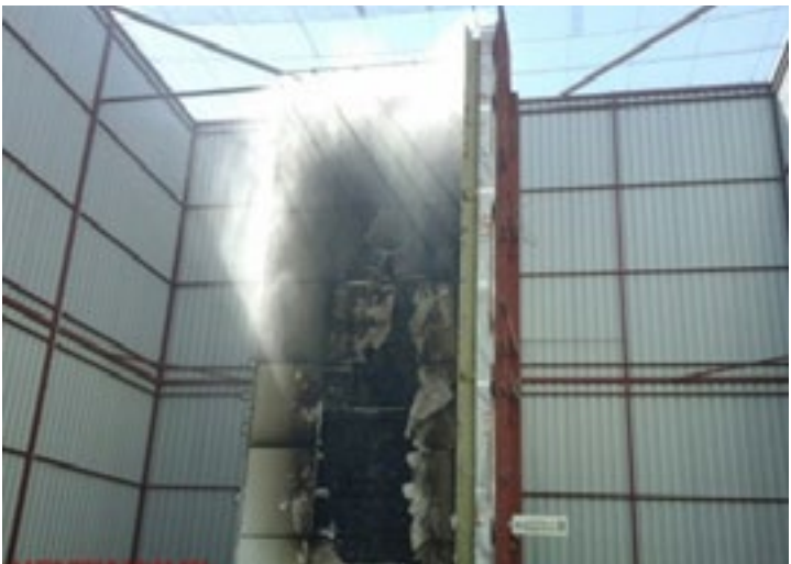
Pic.4 Sprinkler system on. End of test.
